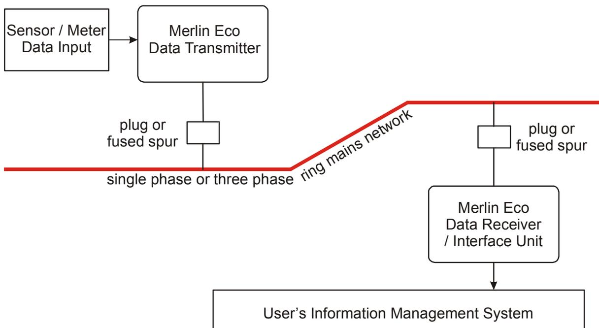
Bi-directional communication can be achieved by specifying the devices to include the capability to both transmit and receive signals.
