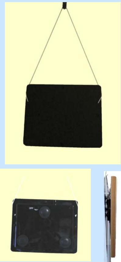
The Model PIC 4 Painting Alarm is a fully portable, battery powered security detector for wall hung objects. It can simply be supported from the same hook or hanging system as the object, and requires little or no setting up. It offers an output to link to a third party alarm system, plus an audible indication at the painting.
